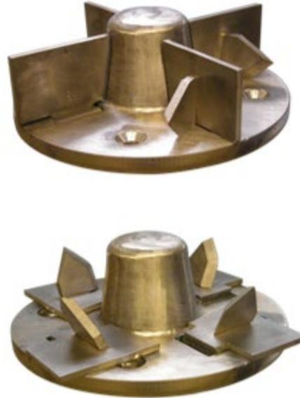
vortex style impeller with hinged vanes that fold flat and expose blades for shredding capability when operated in reverse rotation. Coupled to the variable frequency drive and managed via the smart self-monitoring system, this impeller changes its function when the direction of rotation reverses to cut snarled long fibrous materials and rags, and then removes them without human intervention, or losing its high hydraulic pumping efficiency.
