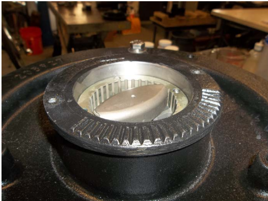
With the housing threaded completely into the suction cover, the shredder cutter bar can be threaded onto the shaft to retain the impeller.
