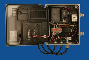
All single phase Fahrenheit® pumps are supplied with a NEMA 4X control box including pump start components, Seal Minder® relay, motor thermal sensor connections, and high temperature wide angle float switch with 20' cable. These single-phase controls meet UL 508A and cUL CSA-22.2 requirements.
