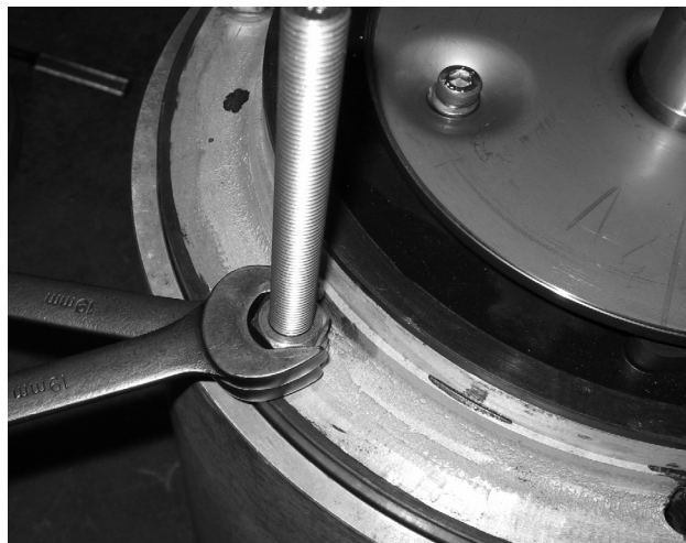
Pic #4 Using two 19 MM wrenches on diffuser nuts
