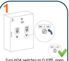
Turn HOA switches to O (Off), open inner door by turning main disconnect to 'Off")
