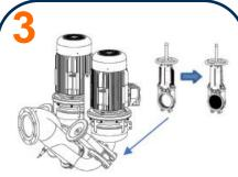
Fully close the branch isolation valve of the motor that will be replaced. The valve or the operational motor must remain open
