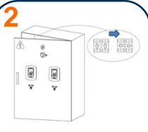
Turn fusible disconnects to the "Off" position. Confirm that there is no power to the motors
