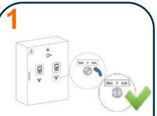
Turn HOA switch to 0 for faulted motor. The operational motor can stay on-line and pumping liquid during this operation (with C-version Body)
