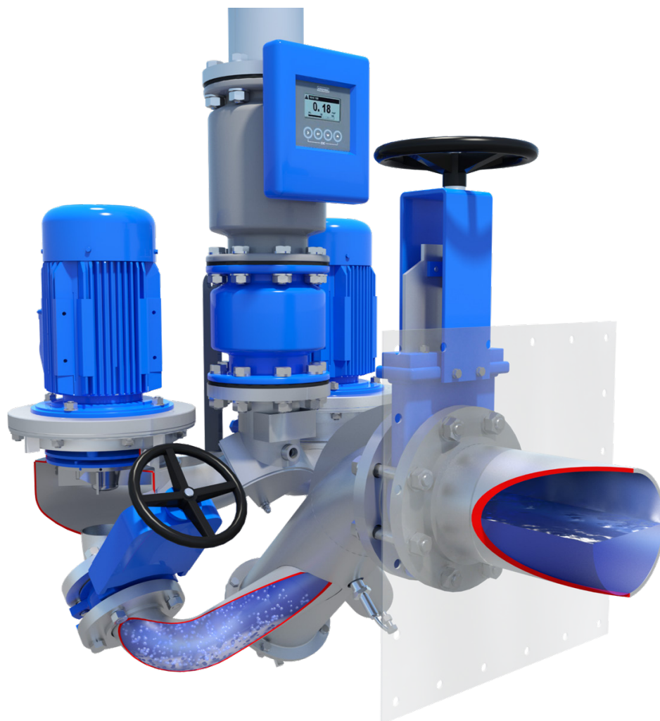
Figure 1: The OverWatch™ system utilizes a duplex pumping system consisting of one 304L stainless steel hydraulic body, two IP67/IE3 immersible motors driven by variable speed drives. One pump is in service while the second pump is in standby.
