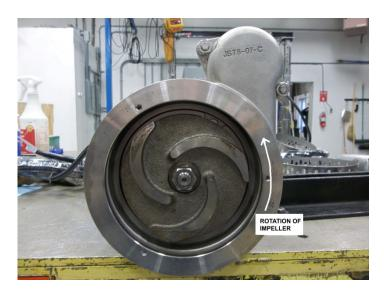
2. By looking from the top of the pump. Since the impeller cannot be seen, the best way to check the rotation is to check the kick back motion of the pump when the pump just starts. The kick back motion of the pump should be counter clockwise as shown in the picture below.
