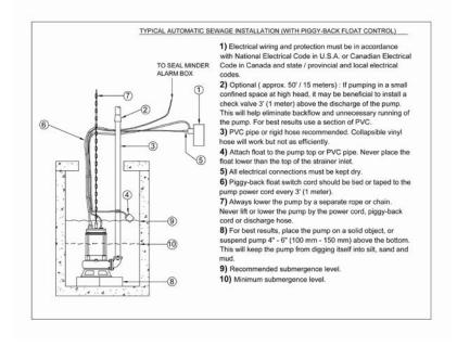
Three phase pumps need a separate control box with float(s) for automatic operation.
