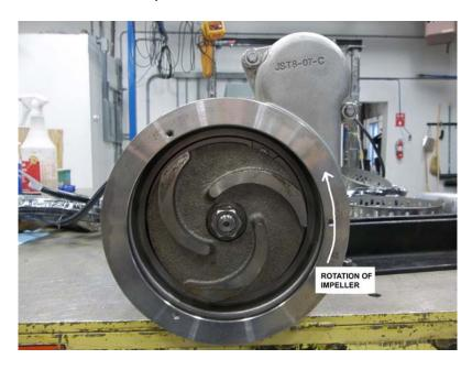
2. By looking from the top of the pump. Since the impeller cannot be seen, the best way to check the rotation is to check the kick back motion of the pump when the pump just starts. The kick back motion of the pump should be counter clockwise
