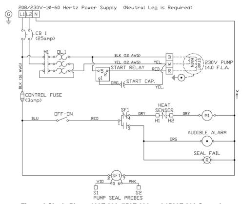
Figure 2 Single Phase 400F-230, 750F-230 and 1500F-230 Control
